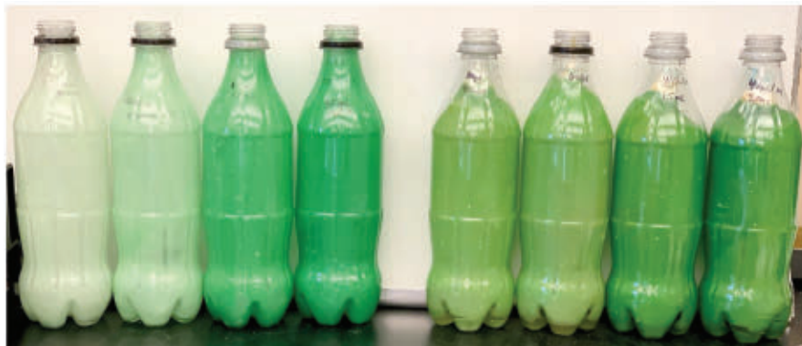
Figure 12. Freshly made samples at 0.5, 1, 2.5, and 5% algae loading levels (left to right) versus the same loading levels after 45 days of storage at room temperature under ambient lights.
