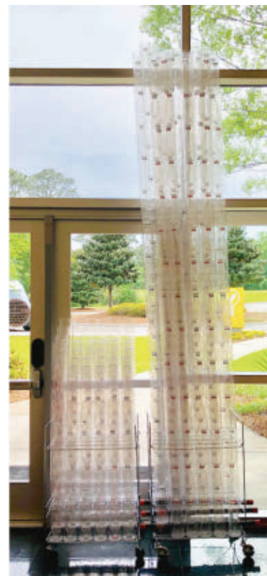
Figure 16. Uncoated PET container proof-of-concept array at 5 containers per sleeve and at 15 containers per sleeve. Because of the ability to vertically scale, within the same floor space “footprint,” the 10-foot-tall array contains 3x the potential coated surface area of the smaller 3-foot-tall array.
