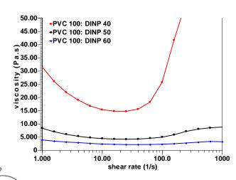
Paste preparations with 40, 50,60 phr DINP. Readings were made 1 h after preparation at 25°C with a Rheometer (TA Instruments, AR2000)
