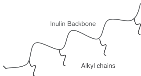
Figure 4.3 Schematic representation of INUTEC ® SPI polymeric surfactant.
