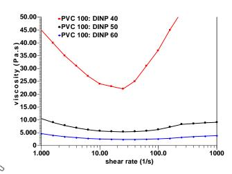
Paste preparations with 40, 50,60 phr DINP. Readings were made 1 h after preparation at 25°C with a Rheometer (TA Instruments, AR2000)
